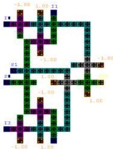
Fig.16. QCA Layout of proposed 4:1 MUX
